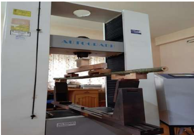
Fig 1. Experimental setup of bamboo sample for bending test
