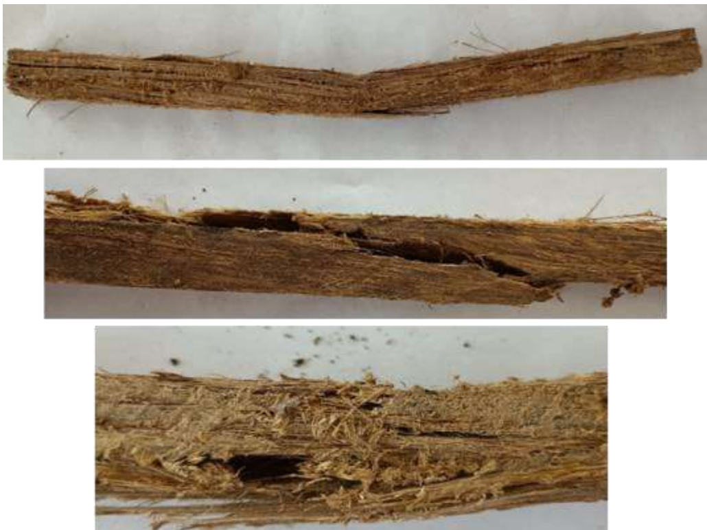
Fig 3. Bending failure modes observed in composite boards. (A) excessive compression failure in the upper-side, (B) Cross grain tension, and (C) Splintering tensions
