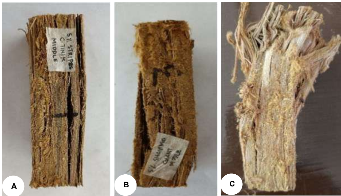
Fig 2. Failure forms of bamboo composite boards after compression test: A. Delamination/splitting failure; B. Splitting with buckling failure and C. Buckling failure
