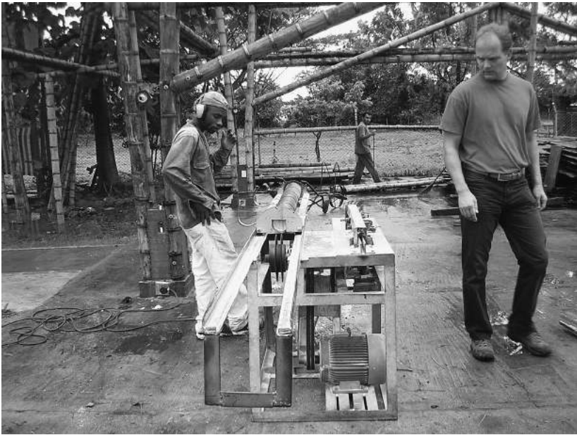
Figure 5. Multi-functional bamboo strip making machine suitable for Guadua designed by Jorg Stamm.
