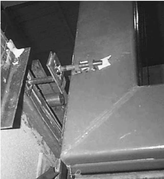
Figure 5. (Top) Photograph of test set-up showing steel frames for lateral support. (Bottom) Photograph of detail of the connection between the loading beam and the lateral support.
