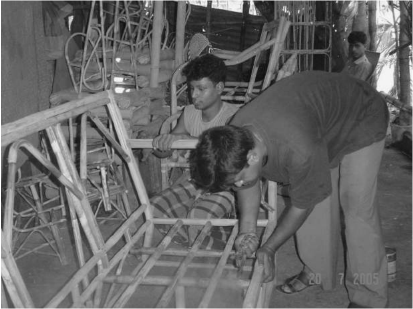
Figure 7. Labor working in a cane industry to prepare a sofa of Chittagong City Corporation area.
