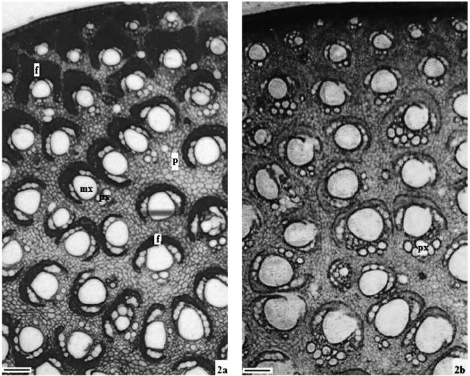
**Figure 2.** Cross-section of *Calamus deeratus*. (a) Basal internode and (b) top internode. Non-uniform and unevenly distributed vascular bundles. Vascular bundles at the periphery and basal internodes have a more extensive fiber sheath than inner vascular bundles and top internodes (f = fiber sheath; P = ground parenchyma; px = protoxylem vessels; mx = metaxylem). Scale bar = 25  $\mu$ m.
