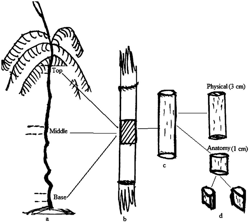
**Figure 1.** Schematic diagram of (a) rattan stem showing three levels: second basal, middle and top internodes, (b) internode showing mid portion (shaded portion), (c) 4-cm-long sample and (d) sample for physical and anatomical investigations.
